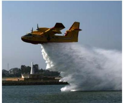
minutes after being requested and drop about 1,600 gallons of water or fire-suppression foam with each pass. They refill their tanks by skimming low over the surface of a lake or ocean. The planes offer peace of mind during the height of fire season.
